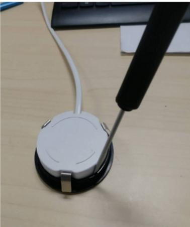
Step 2: Separate the light source and driver.
