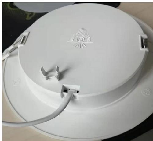
Step 3: LOOSEN THE LED MODULE
