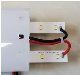
Step 5: Pull out the light source module
