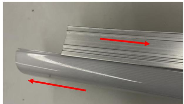
Step 5: Slide out the LED PCB.
